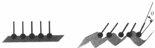
FIGURE 3 Illustration of the LC director alignment along the grooves of the holographic grating written onto the polymer surface
